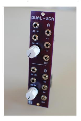
The module is designed and sized for **Eurorack** systems. You will need a 16-10 pin **Eurorack** power ribbon connector with -12/0/+12 which is connected to a synth power supply. You will also need a trimmer adjustment tool, a digital volt meter.
